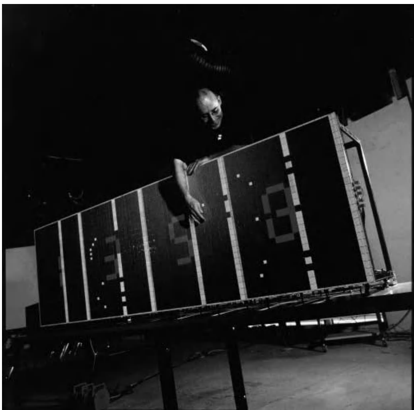
Fig. 14. The present BioWall prototype consisting of about 80 \times 25 = 2000 molecules (Photograph by A. Herzog).
